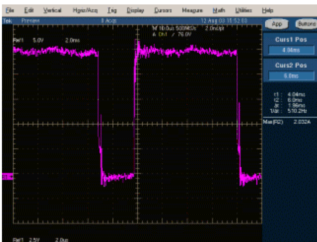
Figure 3-23: Gate signal without a glitch
